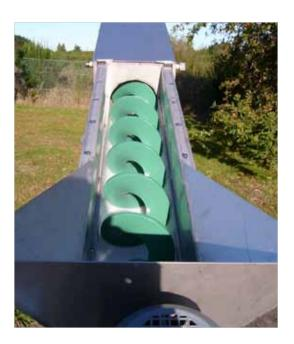
The shaftless auger is made of alloy steel with a protective polyurethane paint. The transport tube is made of 304L or 316L stainless steel with a width of no less than 7" and a thickness of 1/4". High-density polyethylene (HDPE) covers the transport tube to avoid wear.
