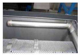
In order to have organics material back in the the wastewater process, 2 spray bars are provided. 1 installed on the conveying part, the other one on the compression box.
