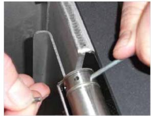
To dewater and compress the debris, the screw will push them onto the lid. To comply with landfill regulation and the Paint Filter Test, the pressure of the lid can be easily adjusted.
