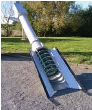
Located at the bottom, a stationary perforated plate basket retains all the debris. Then, a spiral screw convey, dewater, compact and discharge the screenings into a dumpster.
